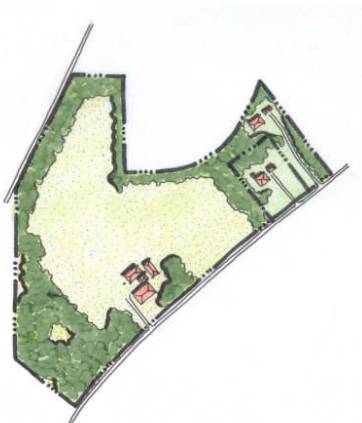
Figure 10: In this approach, the 60-acre parcel was subdivided to carve two 2-acre lots out of a wooded area. Each lot could support a house with its own well and septic system. The farmland was left in a single large field controlled by a single landowner. The farmland could be owned or leased by a farmer.
